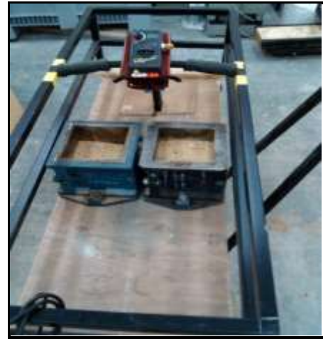
Figure 6: Two sand filled moulds on the machine acting as weights each weighing 20kg
