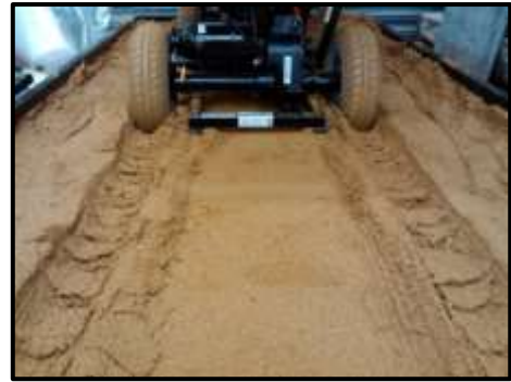
Figure 11: Deepest rut depth illustration in sand bed terrain with the vehicle running on maximum speed, maximum tyre inflation pressure 45PSI and maximum load 800N
