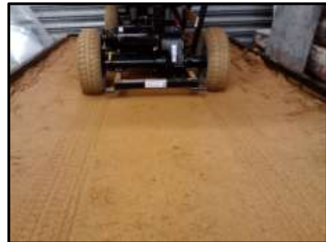
Figure 12: Lowest rut depth illustration in sand terrain bed with the machine running on maximum speed, minimum tyre inflation pressure 3PSI and maximum load 800N
