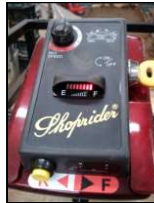
Figure 3: Battery power metre unit
