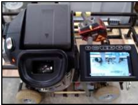
Figure 9: Camcorder fitted to the stand on Mobility SF-3713 to record travel time and wheel slip differences
